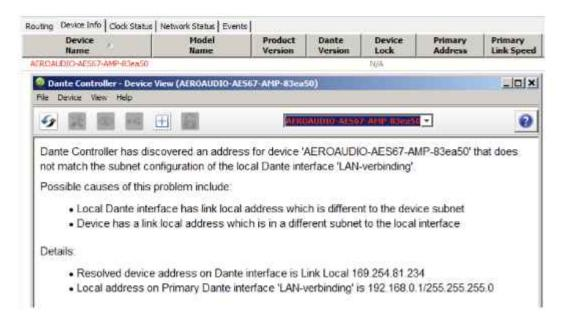
To change setting on the AMP you will need to match the IP address of the computer to the range of the AMP. In this case 169.254.81.xxx
