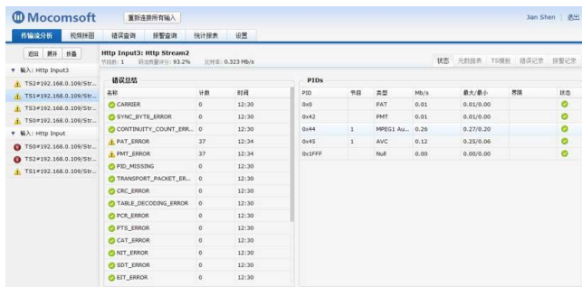
TS layer analysis - TR101 290 errors
