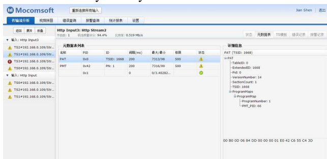
TS layer analysis – PID analysis
